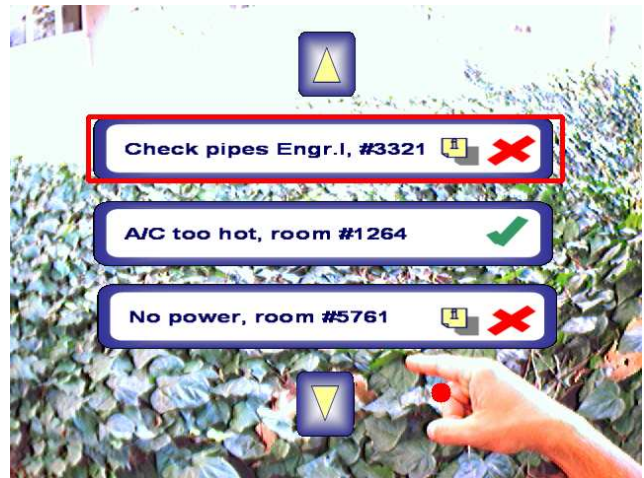
Figure 9: Scrolling through the list of work order summaries. Note that the hand location (big red dot) does not fall on any of the interaction surfaces. Instead, the currently pre-selected item is chosen by discrete postures (“up”/“down” gestures).
