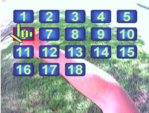
Figure 10: The number selector is operated with registered manipulation. Moving the hand over one of the numbers and performing a selection gesture picks the respective attachment.
