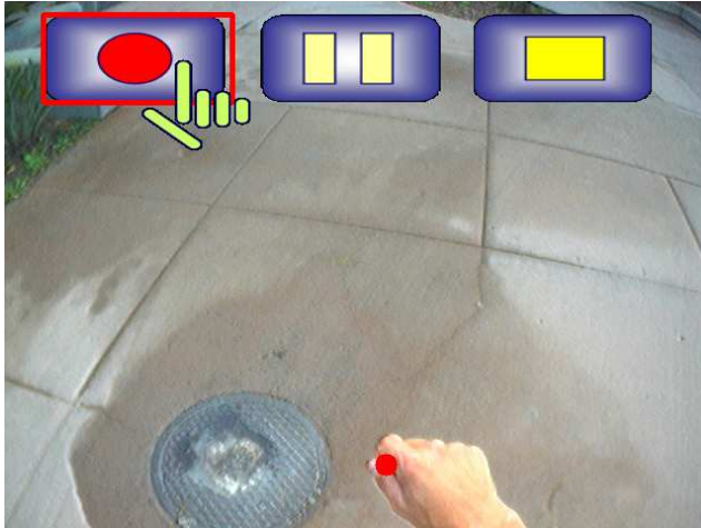
Figure 6: The voice recorder interface in the foreground. Note that the interface snapshots shown in the various figures were taken in different environments, illustrating the ability of our system to adjust to varying backgrounds and lighting conditions. This snapshot was taken while walking.
