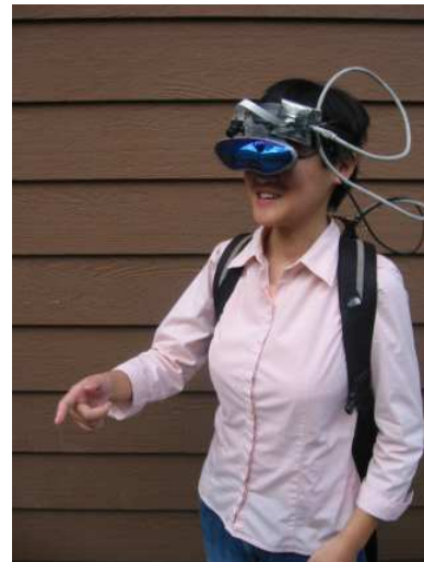
Figure 1: Our mobile user interface in action. All hardware components aside from the display and camera are in the backpack.
