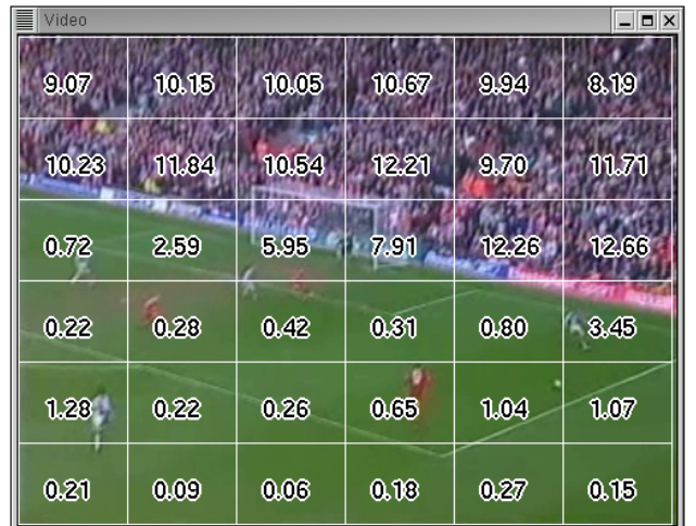
Figure 2: Uniformity metric for different regions of a soccer video. Greater values correspond to less uniform regions.
